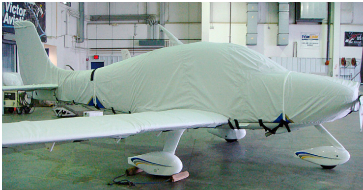
Cirrus SR20 Full Cover Set (Extended Canopy Cover, Engine Cover, Wing Covers, Empennage Cover)
