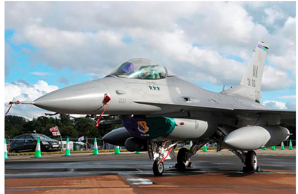
Intake, Maintenance Seat & HUD display covers (Aviano AFB, Italy)
