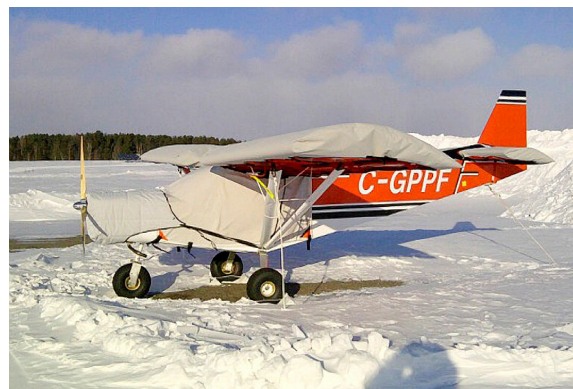
Zenith 701 Canopy, Wing, Tail & Insulated Engine Covers
