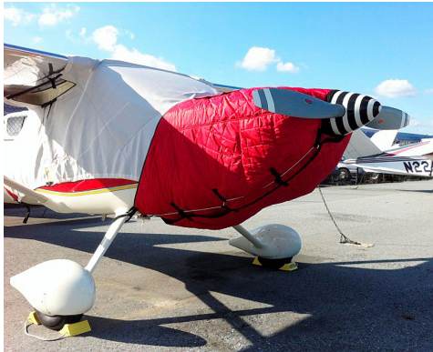
Glstar Insulated Engine Cover
