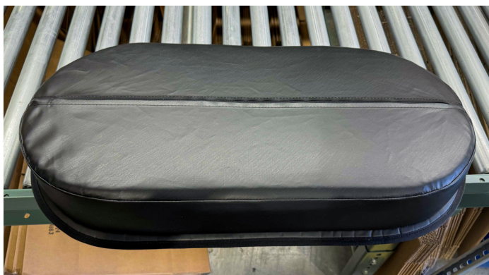
Sikorsky UH60 ENGINE EXHAUST PLUGS (HIRSS type), with safety lip
