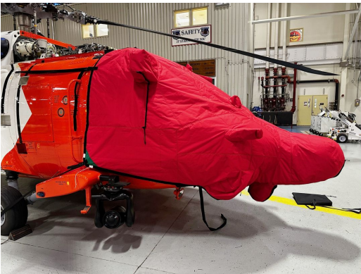
WINDSHIELD/NOSE COVER (HH60G Models: Radar, Refuel Boom & Flir Dome) U.S. Coast Guard MH-60 Cockpit/Nose Cover
