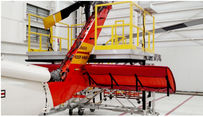
Sikorsky Blackhawk Horizontal Stabilizer Covers, Padded for maintenance protection U.S. Coast Guard MH-60 Padded Horizontal Stabilizer Covers
