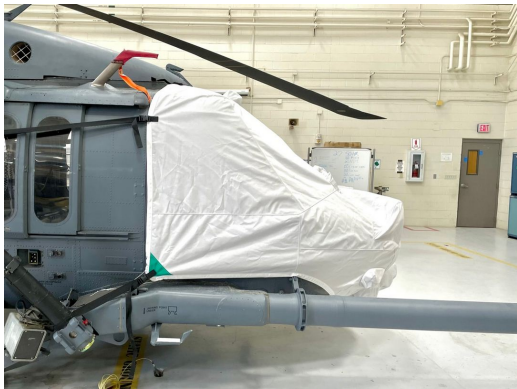
WINDSHIELD/NOSE COVER (HH60G Models: Radar, Refuel Boom & Flir Dome) U.S. Coast Guard MH-60 Cockpit/Nose Cover
