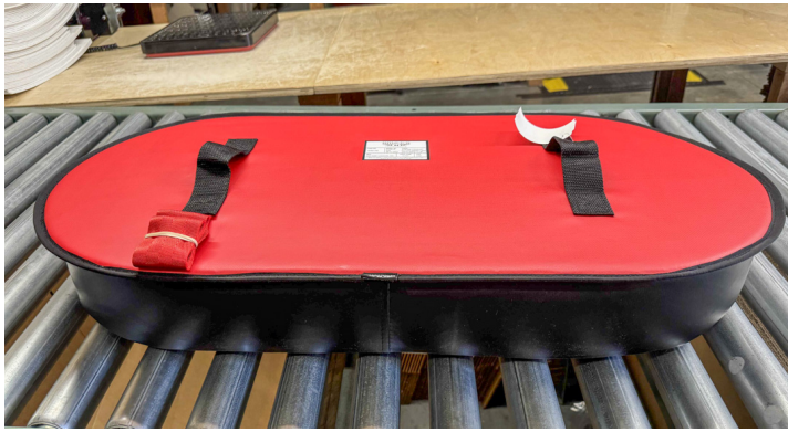
Sikorsky UH60 ENGINE EXHAUST PLUGS (HIRSS type), with safety lip
