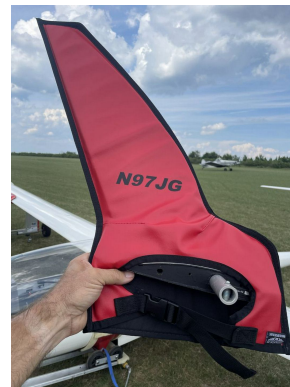
Schempp-Hirth Ventus-2B winglet/wingtip pads
