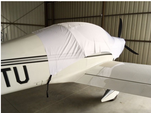
Tecnam Astore Canopy/Engine Cover, test fit cover
