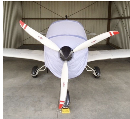
Tecnam Astore Canopy/Engine Cover, test fit cover
