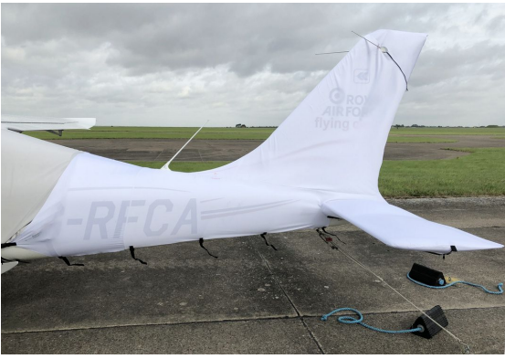
Tecnam P2008 Empennage Cover, test fit cover
