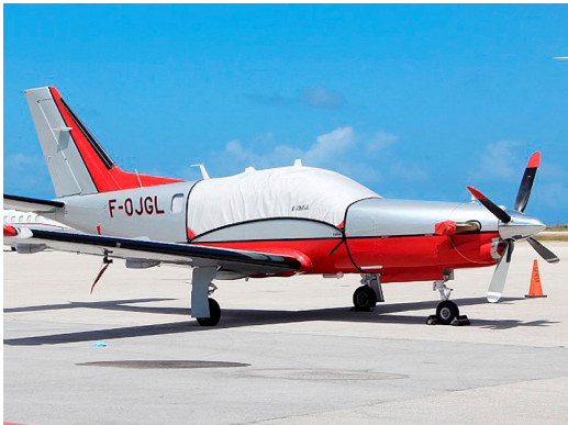
TBM Canopy Cover, Prop Tie/Exhaust Covers
