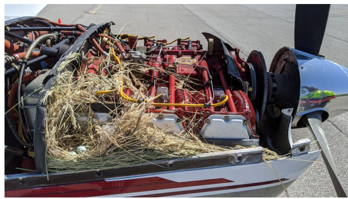
Vans's RV-7 Engine Engine Inlet Plugs ENGINE PLUGS PREVENT BIRD NEST FOD. Piper Saratoga Engine Cowling Bird's Nest
