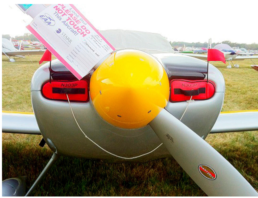
Vans's RV-7 Engine Engine Inlet Plugs ENGINE PLUGS PREVENT BIRD NEST FOD. Piper Saratoga Engine Cowling Bird's Nest
