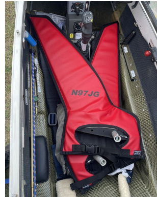
Schempp-Hirth Ventus-2B winglet/wingtip pads
