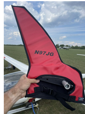
Schempp-Hirth Ventus-2B winglet/wingtip pads
