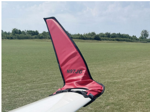
Schempp-Hirth Ventus-2B winglet/wingtip pads
