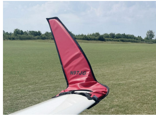
Schempp-Hirth Ventus-2B winglet/wingtip pads
