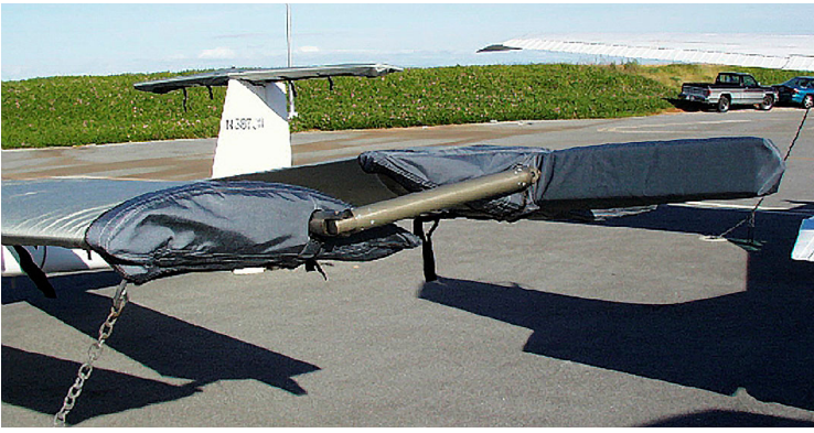
End Cap Covers are used when wing are in folded position. Stemme S-12 Canopy/Nose Cover with Turtledeck Extension, 3D model
