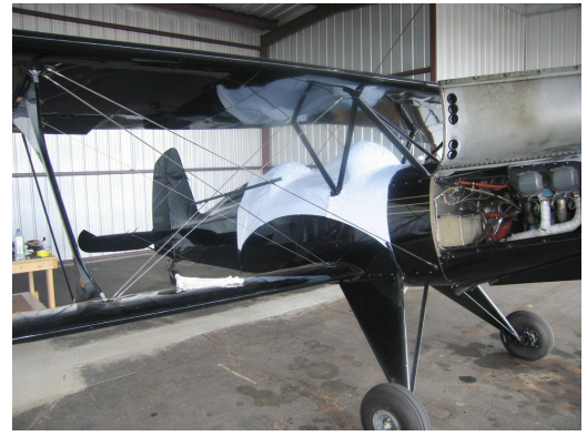
Starduster Too Canopy Cover, test fit cover
