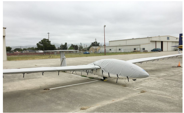
DG-505 Canopy/Nose, Wing, Empennage & Horiz. Stab. Covers
