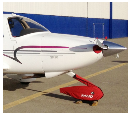
Cirrus SR20 Front Wheelpant/Strut Cover, Engine Plugs
