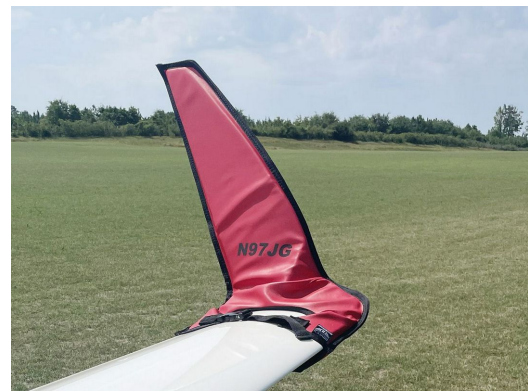
Schempp-Hirth Ventus-2B winglet/wingtip pads
