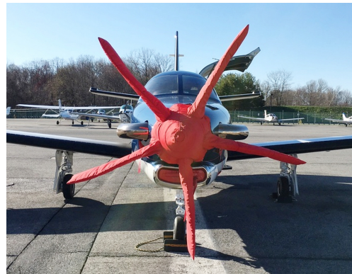
Socata TBM Insulated 5-Blade Prop/Spinner Cover
