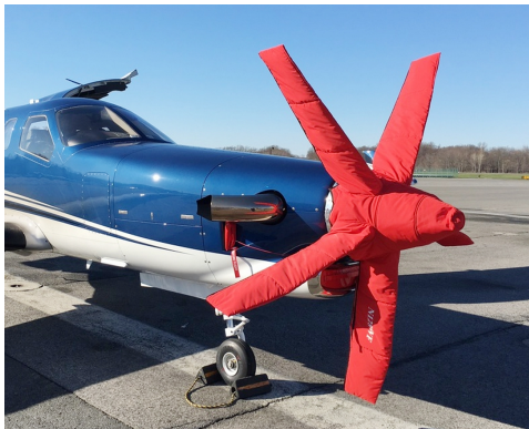
Socata TBM Insulated 5-Blade Prop/Spinner Cover
