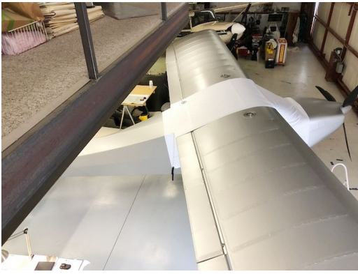
Rans S-20 Canopy Cover, test fit cover
