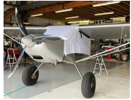
Rans S-20 Canopy Cover, test fit cover
