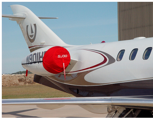
SJ-30 Engine Covers/Exhaust Plug Set
