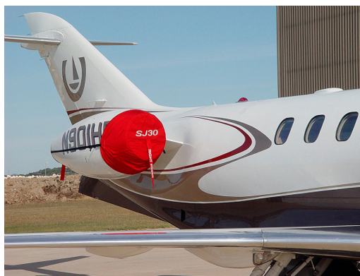
SJ-30 Engine Covers/Exhaust Plug Set
