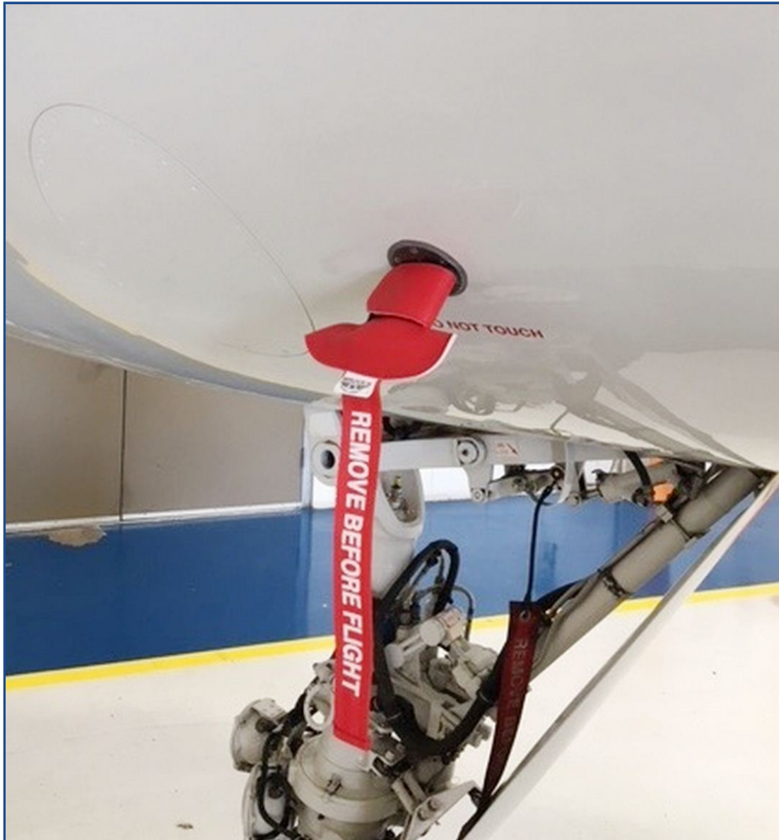
Grumman Gulfstream G-V Rosemont/TAT Cover
