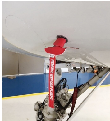
Grumman Gulfstream G-V Rosemont/TAT Cover
