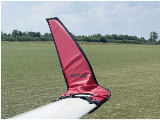
Schempp-Hirth Ventus-2B winglet/wingtip pads
