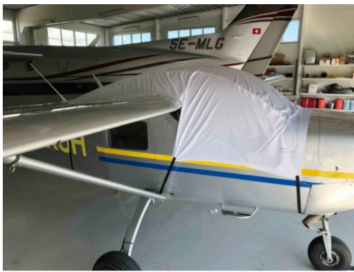
Saab Safari Canopy Cover, test fit cover
