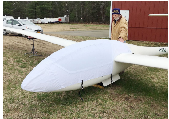
Grob 102 Astir CS Canopy/Nose Cover (test fit)
