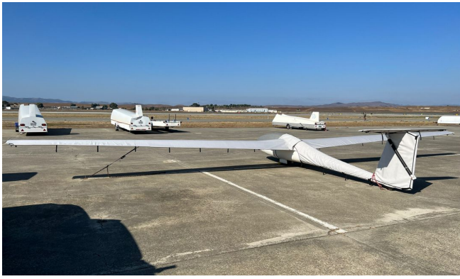
Schempp-Hirth Standard Cirrus Wing & Empennage Covers Schempp-Hirth Ventus 2B Horizontal Stabilizer Cover, test fit cover
