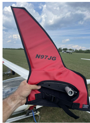
Schempp-Hirth Ventus-2B winglet/wingtip pads
