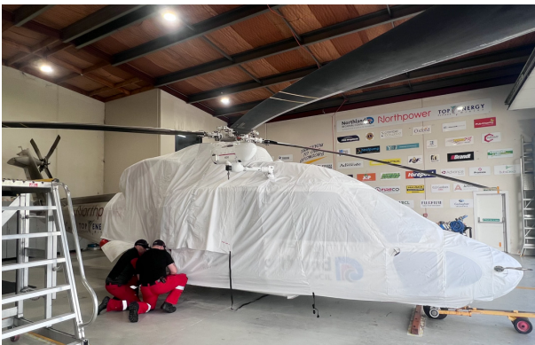
Sikorsky S76C Forward Canopy Cover, Engine Cover (test fit covers)
