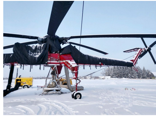
Sikorsky S-64 Skycrane, CH-54 Tarhe Insulated Engine, Rotor Hub, Tailboom, Stabilizer & Tail Rotor Covers
