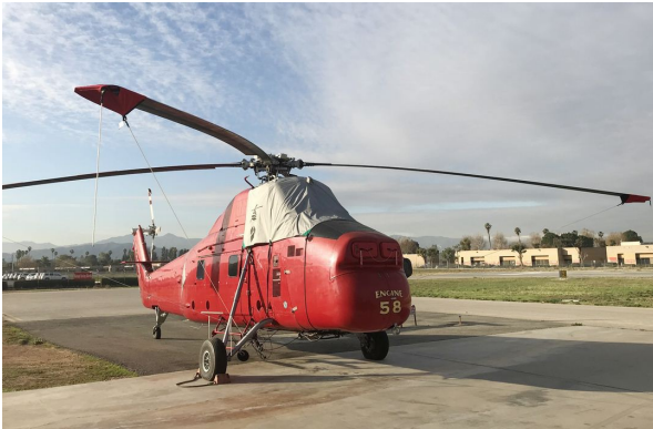
Sikorsky S58T Travel Cockpit Cover, Engine Plugs and Blade Tie-Downs Sikorsky S58T Rotor Hub, Tail Rotor Hub, Engine Plugs, Blade Tie-Downs
