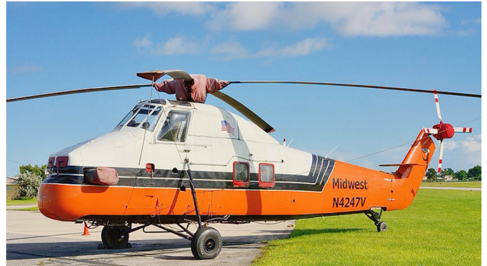
Sikorsky S58T Travel Cockpit Cover, Engine Plugs and Blade Tie-Downs Sikorsky S58T Rotor Hub, Tail Rotor Hub, Engine Plugs, Blade Tie-Downs
