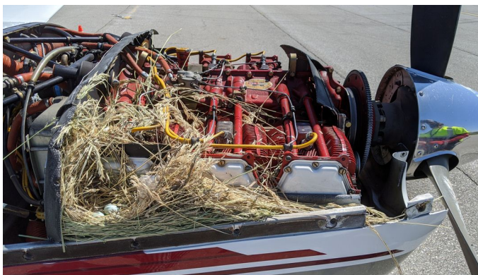
Siai Marchetti SF260 Engine Plugs ENGINE PLUGS PREVENT BIRD NEST FOD. Piper Saratoga Engine Cowling Bird's Nest
