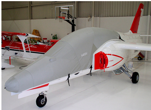
S-211 Canopy/Nose Cover & Engine Plugs
