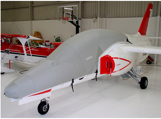
S-211 Canopy/Nose Cover & Engine Plugs
