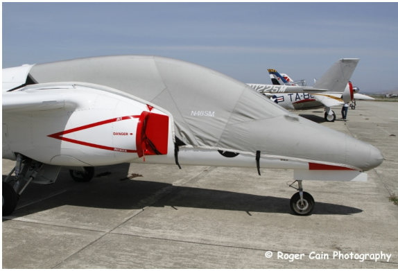
S-211 Canopy/Nose Cover & Engine Plugs
