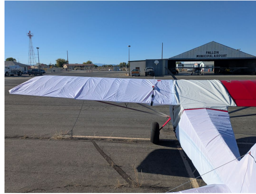
Rans S-20 Raven Canopy Cover, Wing Covers & Empennage Cover (some test fit)
