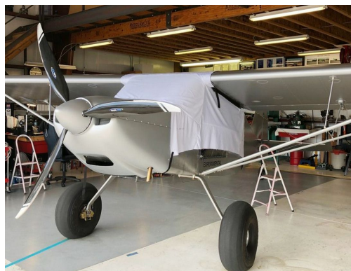
Rans S-20 Canopy Cover, test fit cover
