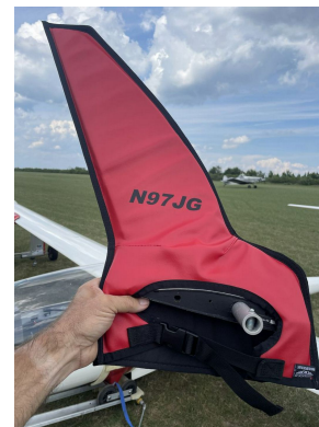
Schempp-Hirth Ventus-2B winglet/wingtip pads
