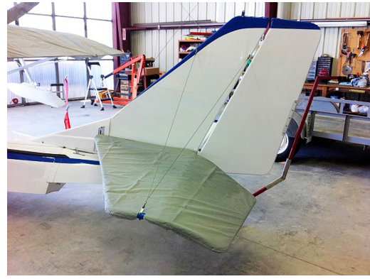
SeaRey Horizontal Stab. Cover (test fit cover)
