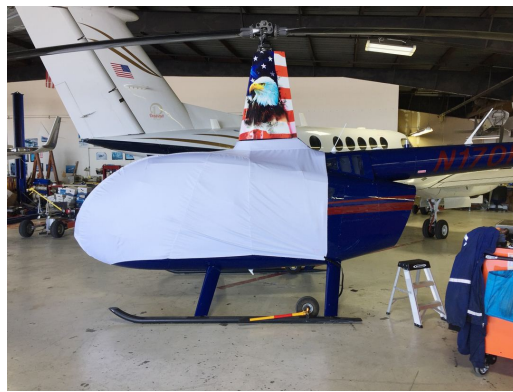
Robinson R-66 Extended Bubble Cover, past rotor mast.
