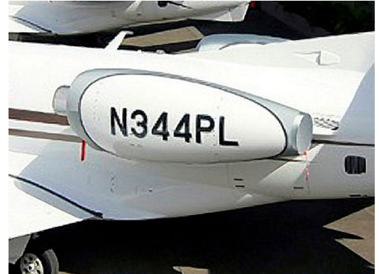
Intake/Exhaust Covers, 3-Strap Type. Successfully installed by two crew, one ladder. Phenom 300 "Bikini" type Engine Cover
