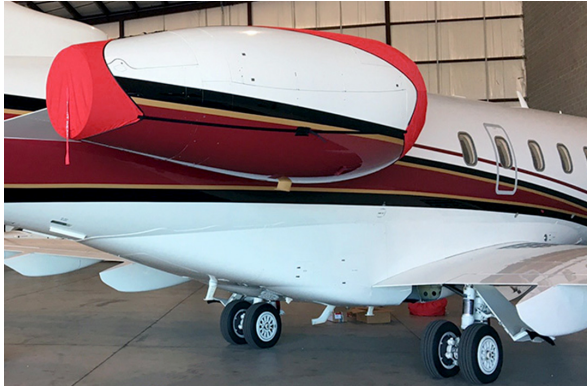
Intake/Exhaust Covers, 3-Strap Type. Successfully installed by two crew, one ladder. Phenom 300 "Bikini" type Engine Cover
