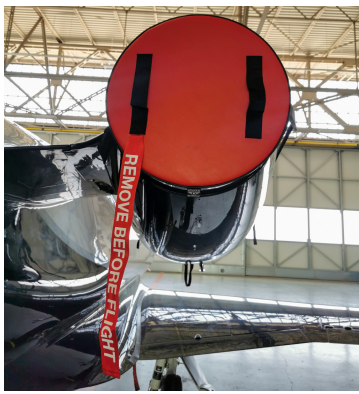
Embraer Phenom 300 ENGINE INLET COVERS & EXHAUST PLUGS (includes lower nacelle plug) (set of 6)
