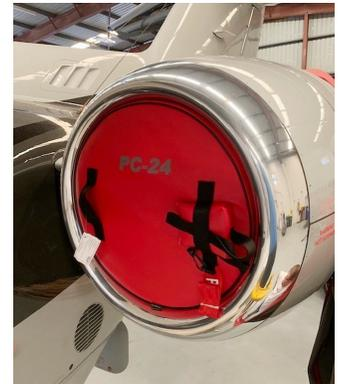
Pilatus PC-24 Engine Intake Plug
