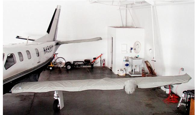
Socata TBM 700, 850 Wing and Horizontal Stabilizer Covers
