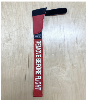
Piper Style Pitot Tube Cover, with Velcro Strap
