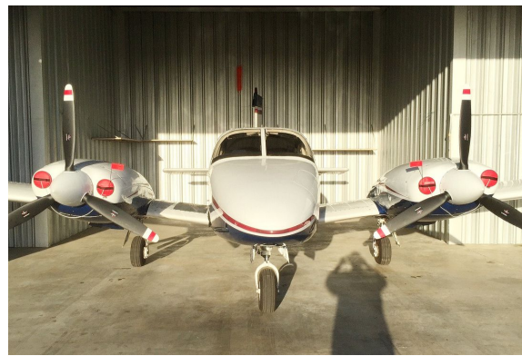
Piper PA-34 Seneca Engine Inlet Plugs (Lopresti Cowling)
