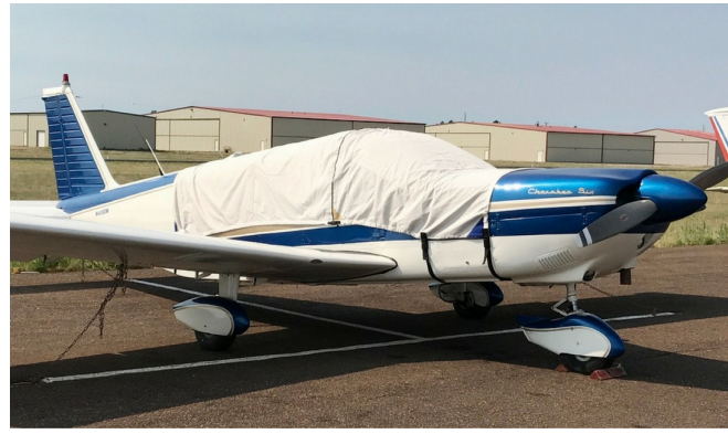
Piper Cherokee Six Canopy Cover with forward bib to cover baggage door.
