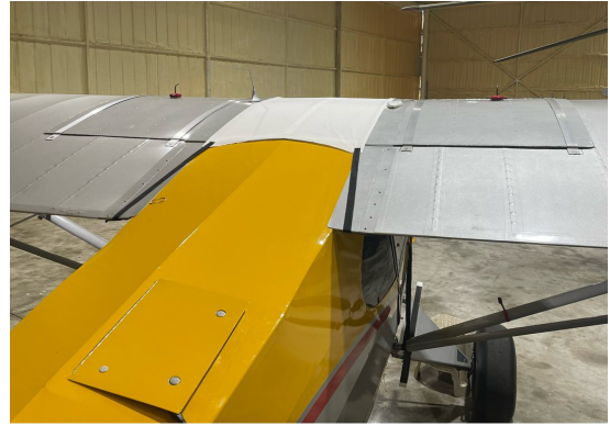
Piper J5A Windshield/Skylight Cover, test fit
