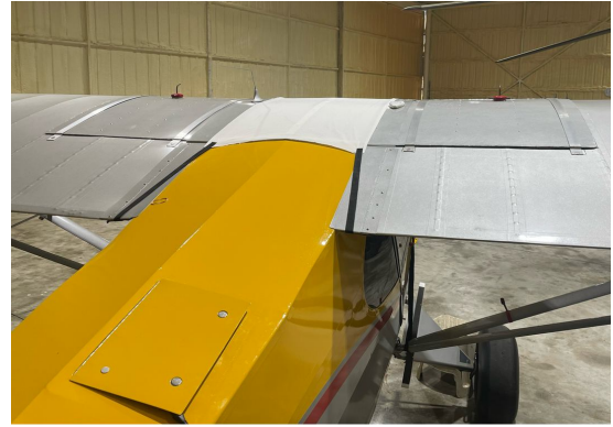
Piper J5A Windshield/Skylight Cover, test fit
