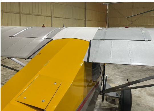
Piper J5A Windshield/Skylight Cover, test fit Piper PA-12 Super Cruiser Canopy Cover (Over-The-Top Style), extended to cover gas caps.
