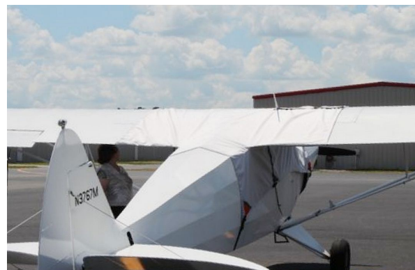
Piper J5A Windshield/Skylight Cover, test fit Piper PA-12 Super Cruiser Canopy Cover (Over-The-Top Style), extended to cover gas caps.
