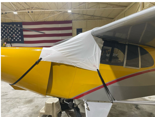
Piper J5A Windshield/Skylight Cover, test fit
