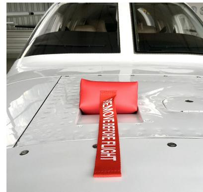
Piper PA46TP-500 Meridian Prop Tie/Exhaust Covers, Engine Plugs Piper PA-46-500TP Engine Cowl Top Plug (Generator Intake)
