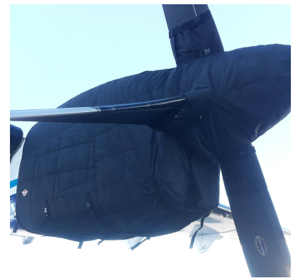
ATR-72-202 Insulated Engine & Prop Hub Covers
