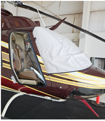
Bell 407 Windshield Cover, pinches into door jambs
