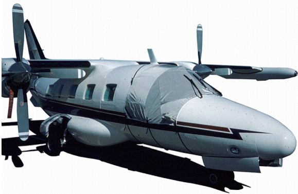
MU-2 Windshield Cover & Engine Plugs
