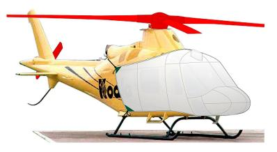
Koala Bubble, Rotor Hub, Blade & Tail Rotor Covers (illustration)
