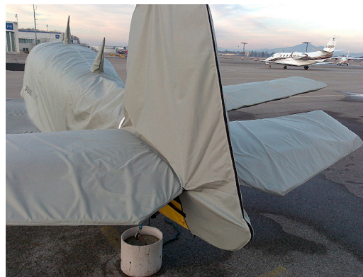
Mooney 231 Full Cover Set: Extra Extended Canopy/Engine Cover, Wing Covers, and Empennage Cover
