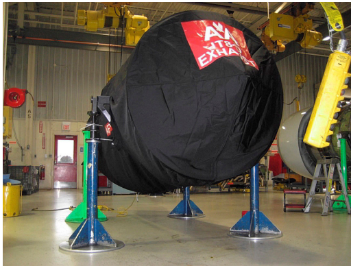
PW JT8D Off-Link Engine Transport Cover (no nose cone, no TR's), fully enclosed
