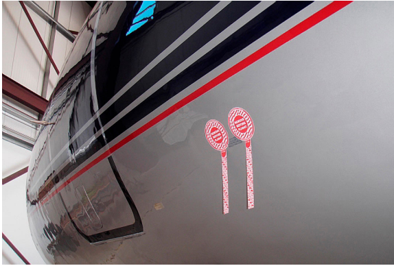
Static Port & Small Inlet/Vent Adhesive Covers: Ideal for Wash Prep and Maintenance
