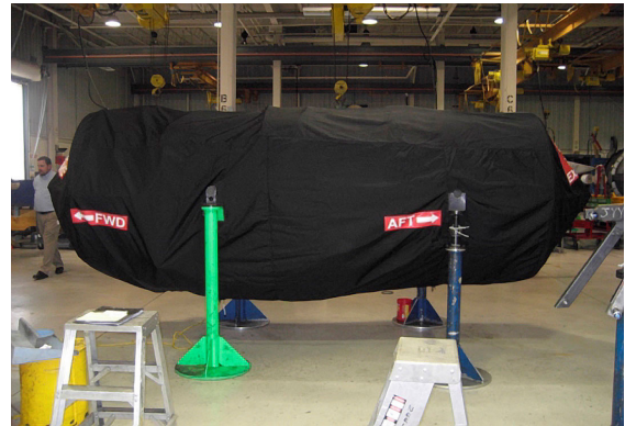
PW JT8D Off-Link Engine Transport Cover (no nose cone, no TR's), fully enclosed
