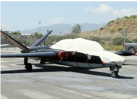
Fougua Magister Canopy/Nose Cover with nose mount loop antenna
