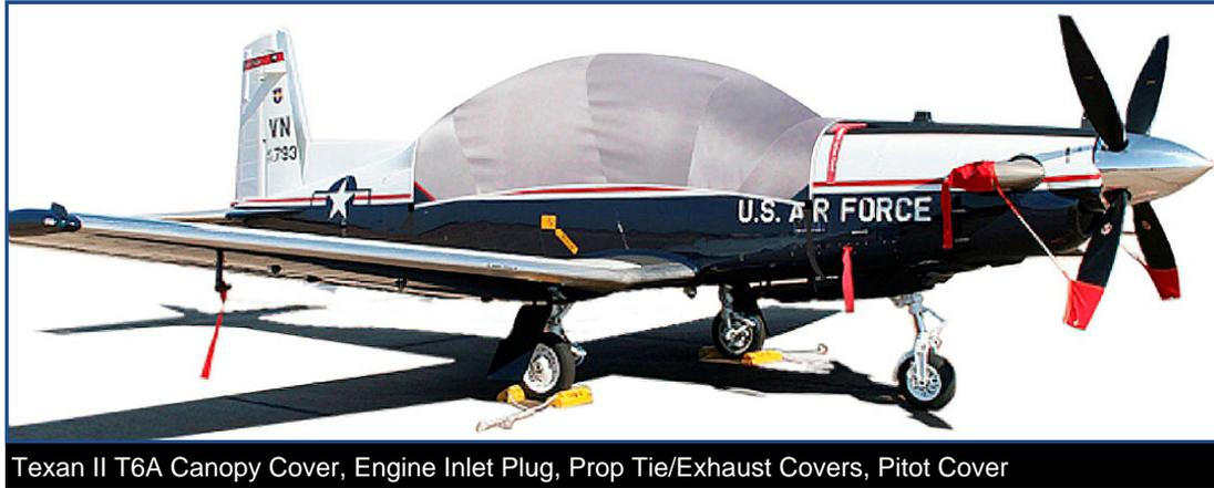
Texan II T6A Canopy Cover, Engine Inlet Plug, Prop Tie/Exhaust Covers, Pitot Cover
